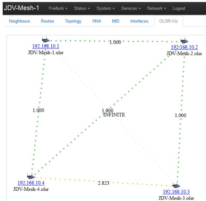
**Gambar 4.2 Skenario pengujian *self-healing***
